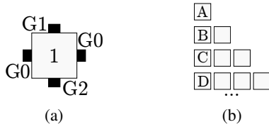
Figure 11: Tile model (a) and a set of possible linear assemblies (A, B, C, D, ...) for the chain assembly experiment (b).
