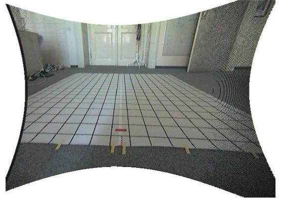
Fig. 3. Image after removing the radial distortion
