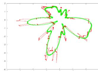
Fig. 1: The raw laser data (red) and data reconstructed using first  $k = 30$  harmonic functions (green).
