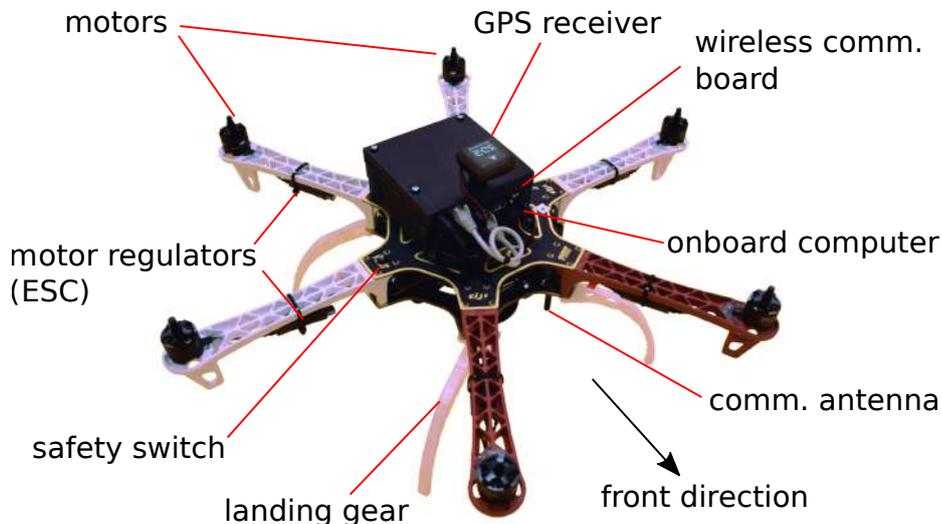
Fig. 2: MUAVET test-bed hexa-copter with propellers dismounted (from [5]).
