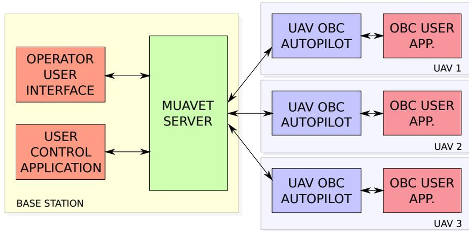
Fig. 3: MUAVET software structure (from [5]).
